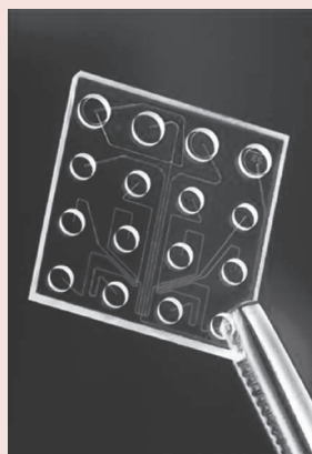
FIGURE 1 Prototype microfluidic channel system developed by Agilent Technologies, which allows 10 electrophoretic separations to be completed in less than an hour in combination with real-time viewing of separations. (Courtesy of Agilent Technologies, Inc., Santa Clara, CA.)
